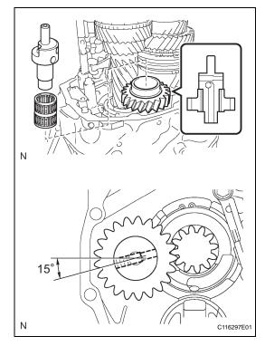
Using a snap ring expander, extend the 2 snap rings and install the output shaft, input shaft, counter gear shaft and control assembly. HINT:
