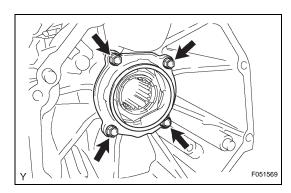
(b) Install the transmission case cover with the 4 bolts. **Torque: 18 N\*m (184 kgf\*cm, 13 ft.\*lbf)**
